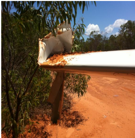
Figure 1: Right wing and nose gear damage
